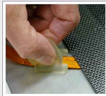
CFRP to metal gaps
