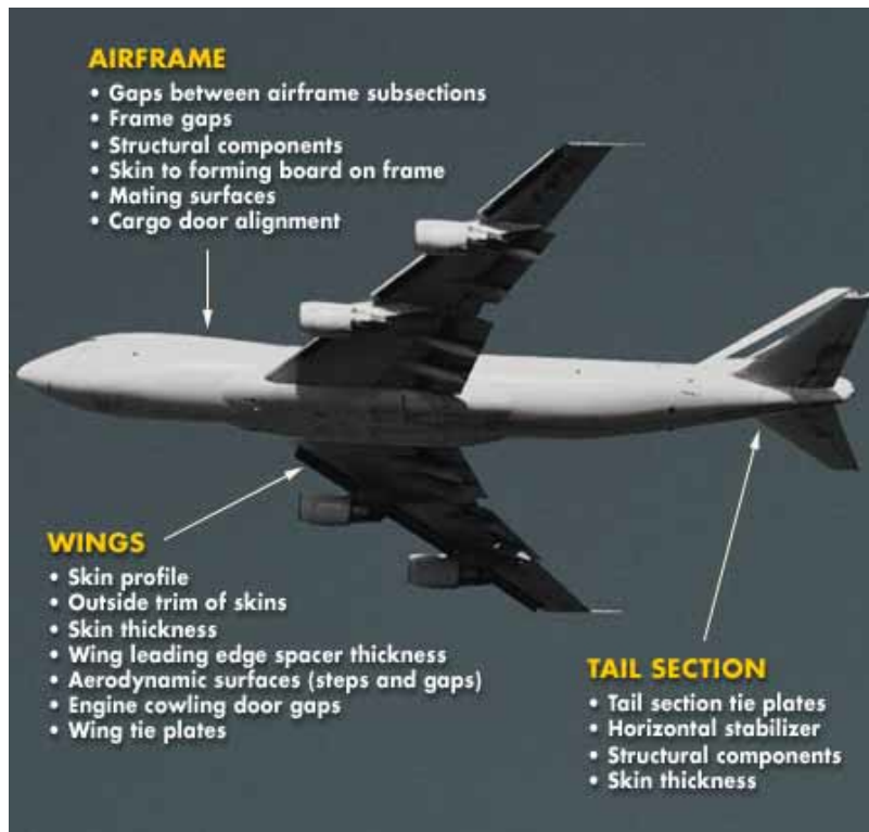
Figure 1: Typical Aircraft gap measurement locations
