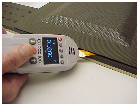
Figure 8: Gapman® Gen3 with integral Flexible Wand measuring very thin gaps CFRP/CFRP
